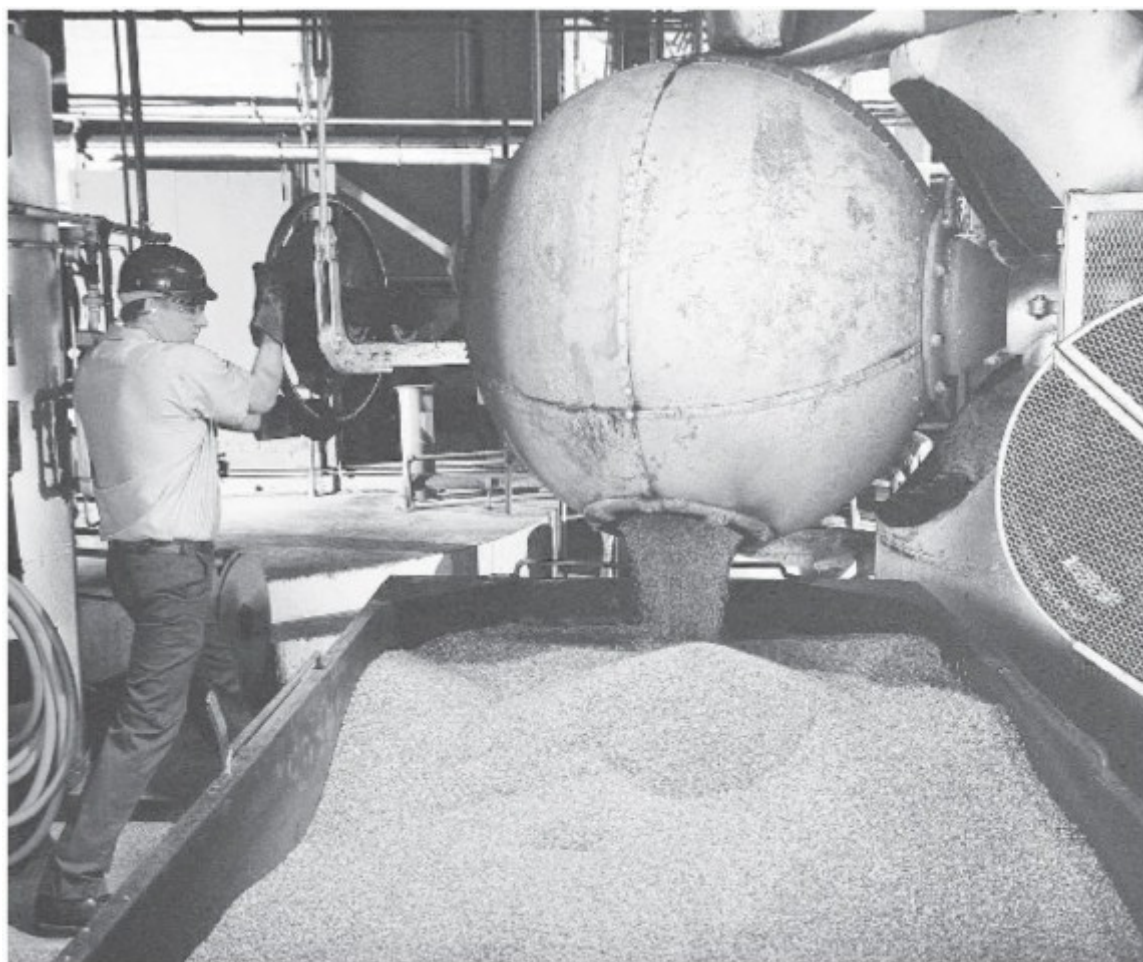
Fig. 5.2: Torra de malte K-Ball em uso na Briess Malt & Ingredients Company. Cortesia Briess Malt & Ingredients Company.
